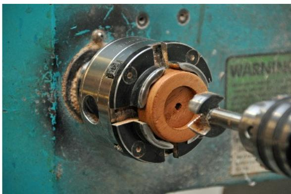
Now turn the axle and wheel assembly. The axle should move freely in the car body without excessive play.
