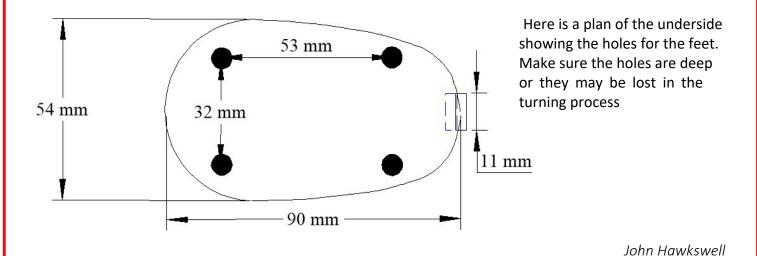
With the blank turned to a cylinder and mounted in a chuck turn the body shape making the rear of the animal slightly heavier. When you have done this drill a 5 mm deep hole in the front to make the snout. Sand and finish the body and part off from the lathe.
