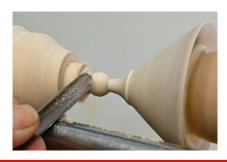
Remember you are working some distance from the chuck so bring up the tailstock for support. The detail gouge can now embellish the stem of the goblet
