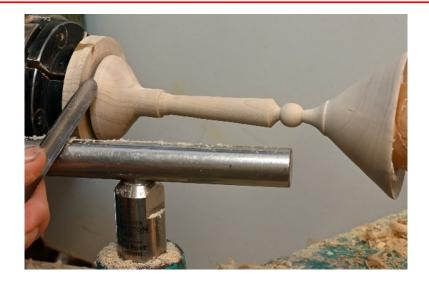
Form the base and then gradually blend in the features on the stem with the detail gouge
