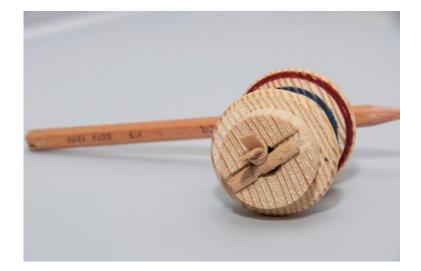
Fit the rubber band at one end. A groove cut in the tank body helps secure the matchstick or turned pin so that it doesn't slip.
