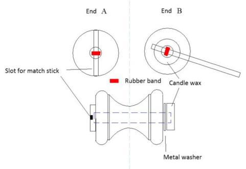
Choose a suitable blank and start by drilling an 7mm diameter hole through the centre.
