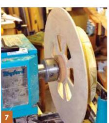
Attach the cycle spindle to one side using M3 stainless steel nuts and bolts. The width of the inner rim now needs to be refined to ensure it is the same as the spindle. Attaching the cycle spindle to one side provides a direct guide to the desired width.
